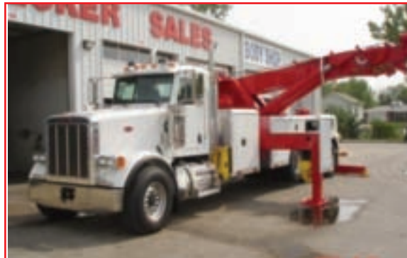
2007 PETERBILT 378 ITS HERE , 565 Cummins, 18 spd, Miller spec chassis, ac, dual chrome exhaust, 20k front axle, alum. wheels, dual polished alum fuel tanks, air lift pusher axle, engine brake, cb-am-fm-stereo, 228" cab to bogie, air ride, cruise, New Century 1075 rotator, 1075S-077-F07, 3 stage recovery boom 75 ton, TOTAL OF 5 WINCHES, 3 underlift, 2-60K winches, 2 spd, 2-20K winches, 1-50K drag winch, 48" alum. tool box, 72" led 16 head light bar, upgrade 8 functions power touch, d-ring options, Hella boom floods, stk#644482
