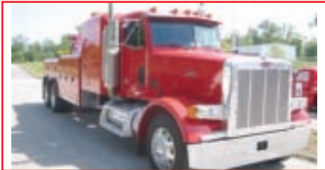
2004 PETERBILT 378 , C12 Cat 430hp, 13 spd, 2 yr 100k engine warranty, 310" WB, 450k miles, ac, Jake brake, Alcoa alum wheels, 60" flat top sleeper, dual chrome exhaust, dual polished alum fuel tanks, New Century 7035, 35 ton boom, 2-35,000lb planetary winches, alum body, hyd. rear spades, code 3 strobe light bar, docking lights, Hella upper floods, tubular light bar, air elec. PTO, manual PTO over ride, air winches free spools, stk#821763
