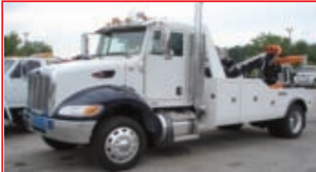
2008 PETERBILT 335 , 335 hp, 8.3 Cummins, 10 spd, air ride, 22.5 alum. whls, tractor package, am-fm-cd-stereo, air suspension dump, VA, VE, Century model 3212 ET, 16 ton boom, 2-15,000lb winches, 84" CA alum. body, 36" alum tunnel tool box, hyd. rear spades, 6K LB tire lift, air winche free spools, 3 PR axle forks, air & electrical hookups, stk#735704
