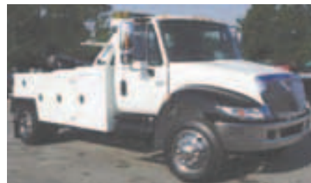
2006 INTERNATIONAL 4300 Stock#307253, DT466 255 hp engine, 6-speed transmission, 31,000# GVW, air conditioning, Vulcan model V-30, 16-ton boom, 2-15,000# winches, 36" stainless steel tool box, 84" stainless steel body.
