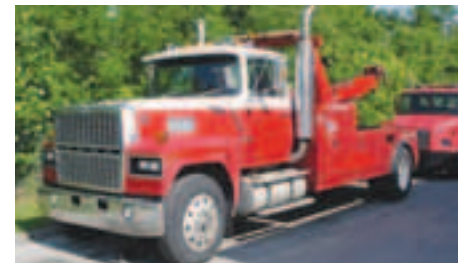
1988 FORD LTL 9000 Stock#009286, 310hp 3406 CAT, 15-speed transmission, 240" wheelbase, odometer shows 3300,284, Century 925, 25-ton boom, 2-25,000# winches, 136" ca steel body, hyd spades, hdu underlift
