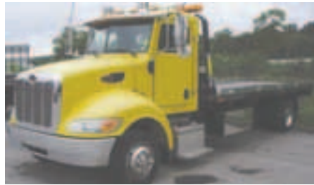
2005 PETERBILT 335 Stock#856371, C7 CAT diesel engine, 6-speed transmission, spring suspension, air compressor on motor, Jerr-Dan 21' steel carrier, aluminum removable rails, 8,000# winch, 2 steel tool boxes with stainless steel fronts, upper floods.
