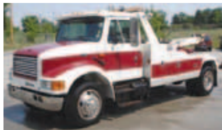
1999 IH 4700 Stock#206762, DT 466, 7-speed trans, 25,500 GVW, air conditioning, Vulcan model 896, Serial#896 00503, 12-ton boom, 84" steel body, 24" tunnel box, 2-12,000# winches
