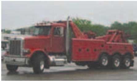
2003 PETERBILT 378 Stock#584643, featuring a C-15 475 hp CAT diesel engine, 10-speed transmission, 399,000 miles, air ride suspension, Century 9055, 50-ton boom, 3-stage boom, 50,000# planetary winches, low rider underlift with 156" reach.
