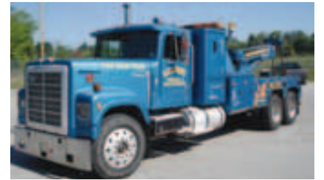
1983 IH 9370 Serial#B11523, 350 hp Cummins, 9-speed transmission, 50,000# GVW, 38,000# rear spring suspension, 1988 Challenr 6800 T-1, Serial#W39100488, 35-ton recovery boom, 2-30,000# winches, air winch free spools, cable tensioners
