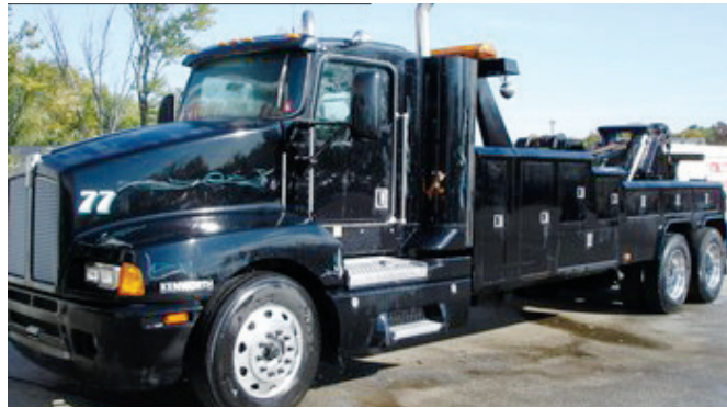
1999 KENWORTH T-600 Stock# 816460, 460hp n14 Cummins, 13-speed, 54,000lb GVW, 14,000# steer axle challenger model CH30, serial# ch30t35 0122f99, 30-ton boom, 2-35,000# planetary winchs, air winch free spool, 116" reach 3-stage underlift
