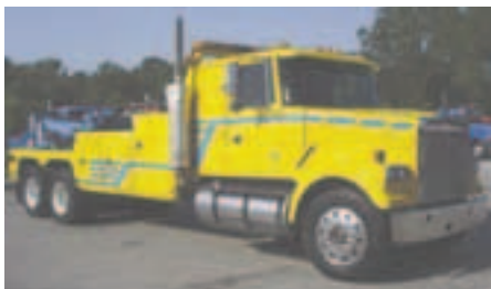
1987 VOLVO WHITE Stock#120537, featuring a 430 Cummins diesel engine, 8-speed transmission, Jake brake, air ride suspension, NoMar Model 2025, 25-ton boom, (2) 25,000# winches, HD tow bar and Whelen strobe light bar.
