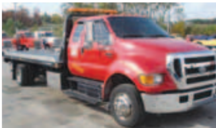
2004 FORD F650 Stock#614732, 3126 CAT diesel, automatic transmission, 151,800 miles, AM/FM CD player, Jerr-Dan 21' steel shark, Serial#21slpb 35105, 10,000# deck, 8,000# planetary winch, cable roller guide, federal amber light bar
