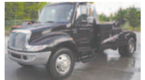
2004 INTERNATIONAL 4300 Stock#651201, 250 hp DT466 engine, 6-speed transmission, 29,200# GVW, air brakes, Vulcan model 897, 14-ton boom, 2-14,000# winches, 36" tunnel tool box, remote winch free spools, Federal light bar.
