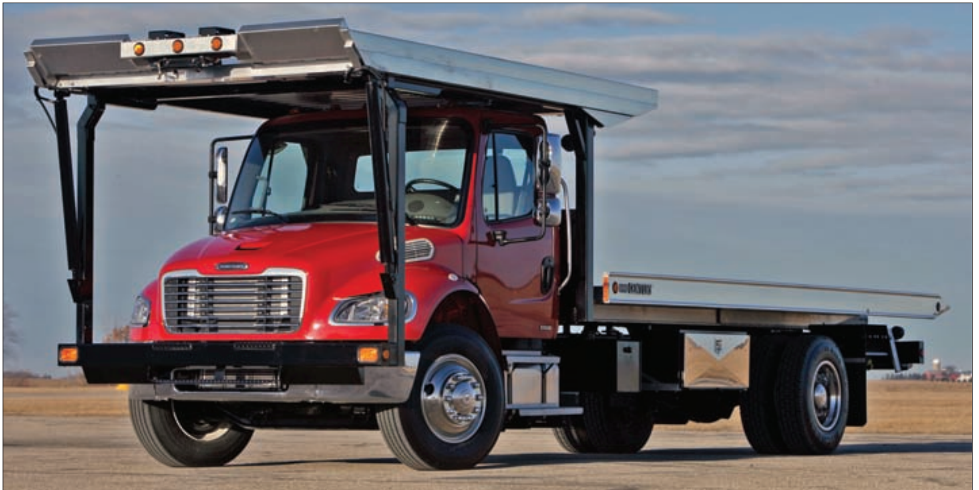
Zip's Freightliner M2 automatic with a Century 22-foot aluminum carrier
