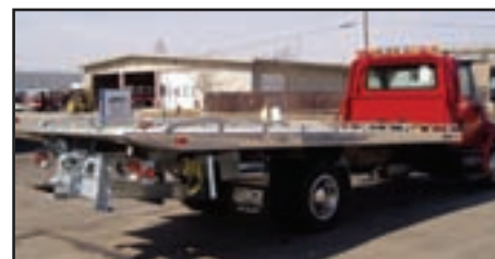
2432C 2007 IH 4300 Century 21' Aluminum Carrier DT466, Auto, Power Windows, Locks, Mirrors, Tilt, Cruise, Air Seat. Aluminum Carrier w/8 Key Slot Package, Removable Rails, Pivoting L-Arms Galvanized Sub-Frame, Hot Shift PTO
