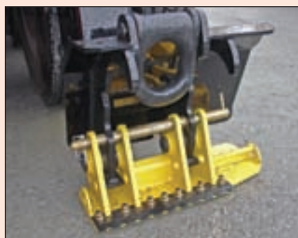
New multi-positional flipper foot option
