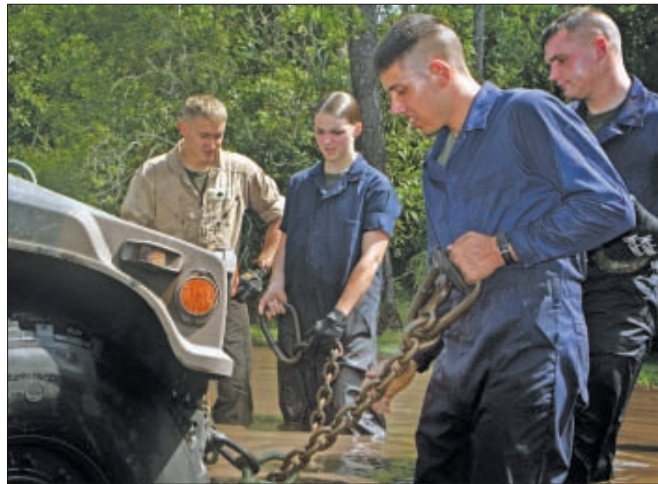
Marines from Motor Transport Company, II Marine Expeditionary Force Headquarters Group, Camp Lejeune, N.C., attach chains and shackles to the tow hooks of a Humvee. This training is preparation for a scheduled six-week Vehicle Recovery Course at Fort Leonard Wood, MO. The chains will be attached to an MK36 medium tactical wrecker to drag the Humvee out of the swamp.
