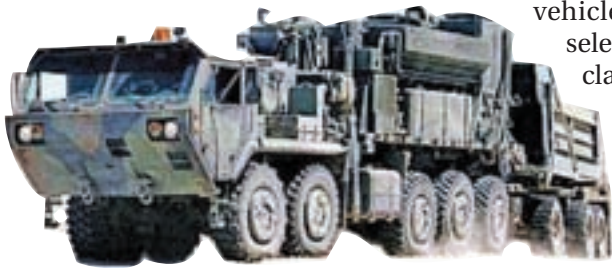
The Army's Palletized Load System (PLS) used as recovery vehicles in Iraq
