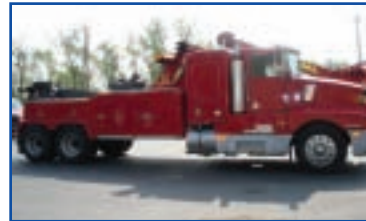
1986 Kenworth T600A #U-2213, NTC 350 Cummins, 9 SPD, Red/Silver, 44" Sleeper, Vulcan 3025 Integrated, Hydraulic Spades, T/L, U/L, 278" WB. $$$$$$
