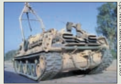
An M88A2 Hercules weighs 70 tons fully loaded and has the capacity to lift 35 tons
