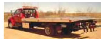
295843 - New 2008 Ford F-650 Jerr-Dan 21' Aluminum Removeable Rail, SRS10 Side Recovery System, 8000 lb Worm Gear Winch, 3500 lb. Wheel Lift.
