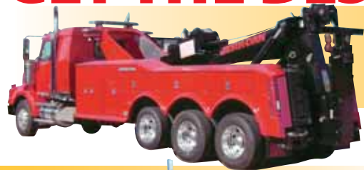
278939 - 2008 Sterling Bullet Jerr-Dan 40 MPL Wrecker Dual Line Tow Sling, 8K lb. Dual Work Gear Winches, 8 Ton Integrated Boom-64" Reach.
