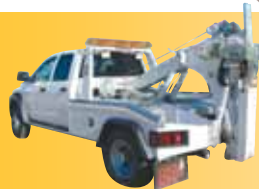
278939 - 2008 Sterling Bullet Jerr-Dan 40 MPL Wrecker Dual Line Tow Sling, 8K lb. Dual Work Gear Winches, 8 Ton Integrated Boom-64" Reach.
