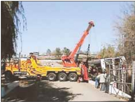
Rolling this tanker back and re-loading it by using the boom on the NRC in the rearmost position shows why the slider feature is so important. The operator is using four winch cables to ensure full load control.
