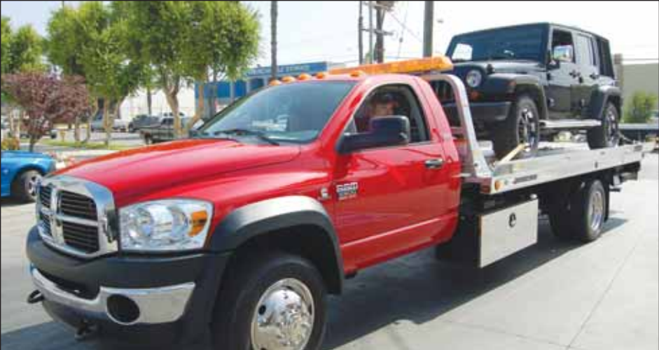
The 2008 Dodge Ram 5500 Chassis Cab has a maximum GVWR of 19,500 pounds. The Gross Combined Weight Rating (GCWR) for both 4500 and 5500 models is 26,000 pounds.
