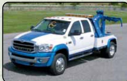
Sterling Bullet 4500 Cummins 305HP Auto w/Chevron Renegade Twin Line Wrecker
