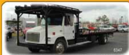
1998 Freightliner FL-70 • 250HP CFE-250HT Engine • 6SP Eaton Fuller Transmission • AC/PW/CC • Jake Brake • Air Ride Driver Seat • Aluminum Wheel Simulators • Tilt/Tele Wheel • (2) 32" Steel Toolboxes • (1) 48" Steel Toolbox • 75 Gallon Fuel Tank • 45 Gallon Fuel Tank • Collins Dollies Attached • 3-way Switch Panel • Jerrdan 28" Steel Rollback • 4 Work Lights • 2 Tail Light Housing • Air Shift PTO • 96" Bed Width
