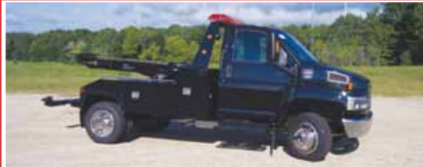
2006 C5500 DURAMAX, AUTO, LOADED CAB, 19,500 GVW WITH A VULCAN 882 WRECKER, 24" TUNNEL BOX, BOTH WITH STAINLESS STEEL OPTION, STOCK #T4492
