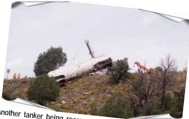
The tanker is almost to the top of the canyon near the roadway just prior to setting it on the roadway. We used an NRC Rotator and one Century 9055 50-ton to recover this wreck.
