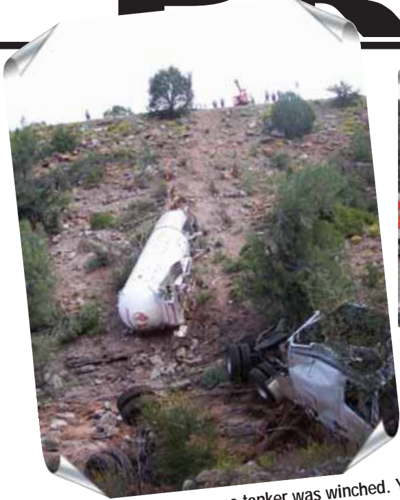
The tanker is almost to the top of the canyon near the roadway just prior to setting it on the roadway. We used an NRC Rotator and one Century 9055 50-ton to recover this wreck.
