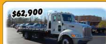
2008 Peterbilt 325, 240 HP Paccar Engine, Allison Automatic, Chevron Series 10 Rollback, Ramsey Worm Winch, Federal Signal LED Light Bar, 96" Bed Width, 2 In Rubber Work Lights, LED Lights
