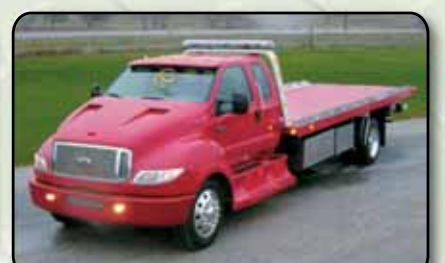
Ford F650 Super Cab 260HP Auto w/Extreme Magna Pro Star & Chevron 21' Steel Carrier
