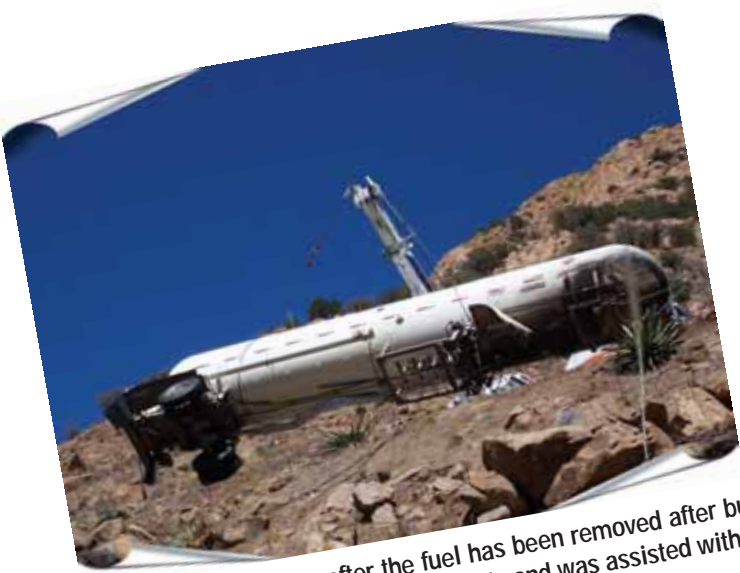
This shows the distance one tanker was winched. You can see what is left of the tractor. One tow truck is visible on the right side and the other tow truck is behind the tree. Both trucks were used and the tanker was winched to the top and ended up directly between the two tow trucks. The tanker was then picked up and placed on the roadway.
