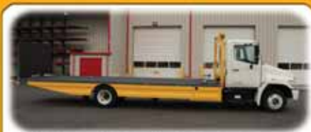
2008 Hino, JO8E-TV 220 HP Engine, Auto Trans, AC/PW/PL/CC, Jones Body Rollback, Top Deck Grit Coated, Monarch 3035 Electric Motor and Hydraulic Pump, Single Piece Tailgate Ramp, LED Light Bar, 12 K Winch, Toolbox
