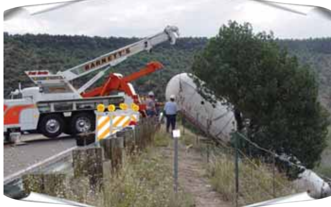
The tanker is almost to the top of the canyon near the roadway just prior to setting it on the roadway. We used an NRC Rotator and one Century 9055 50-ton to recover this wreck.
