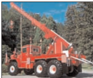
1987 GMC General , 350 Cummins, 9 spd., p/s, a/c, electric windows, aluminum wheels & tanks. Century 20 ton wrecker w/hyd. Jacks, 220 w/b. Very Nice Condition. $ 24,250 OBO Call (859) 441-2200
